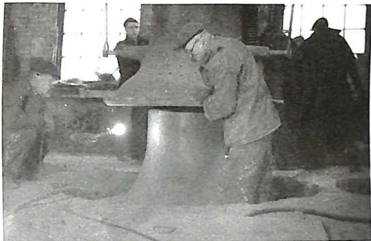
Closing the molds. The "case" is dropped over the "core." Special care has to be taken that the two molds, which weigh as much as the bell itself, are not bumped together during this process.
