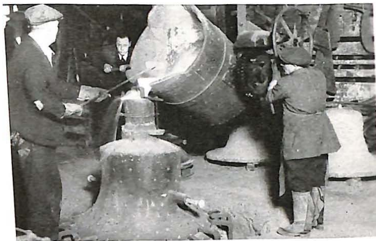
"Pouring" the bell. The metal has been melted and mixed into the alloy in a furnace.
